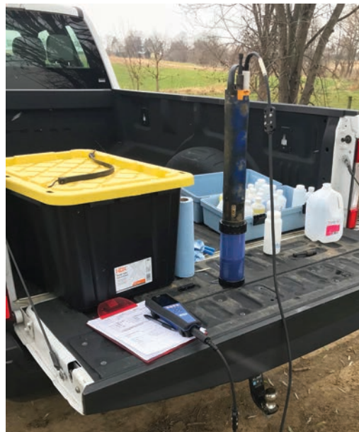
In field calibration of a Sonde unit located within the Mill Creek watershed.
