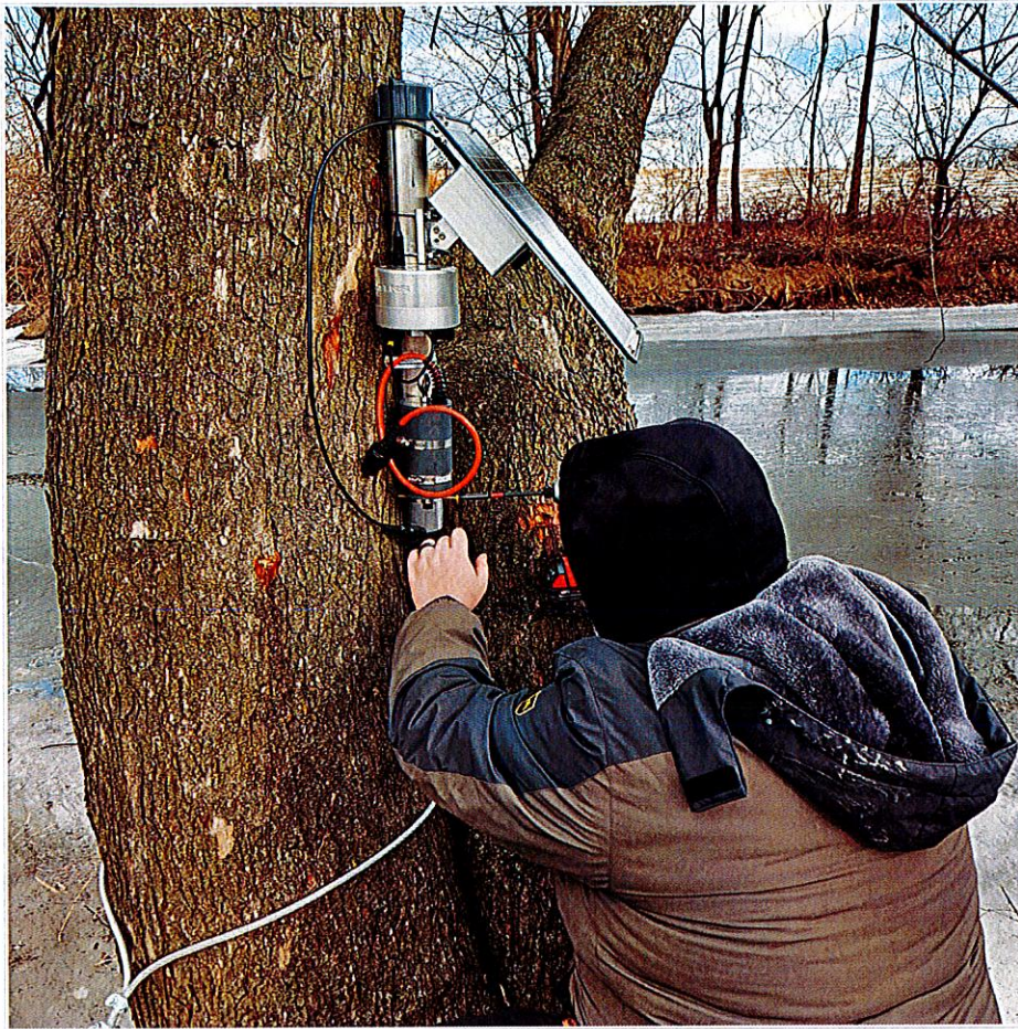
Tyler Keefer installing an X3 telemetry unit along the upper Conestoga River. (Credit: Amanda Goldsmith / LCCD)
