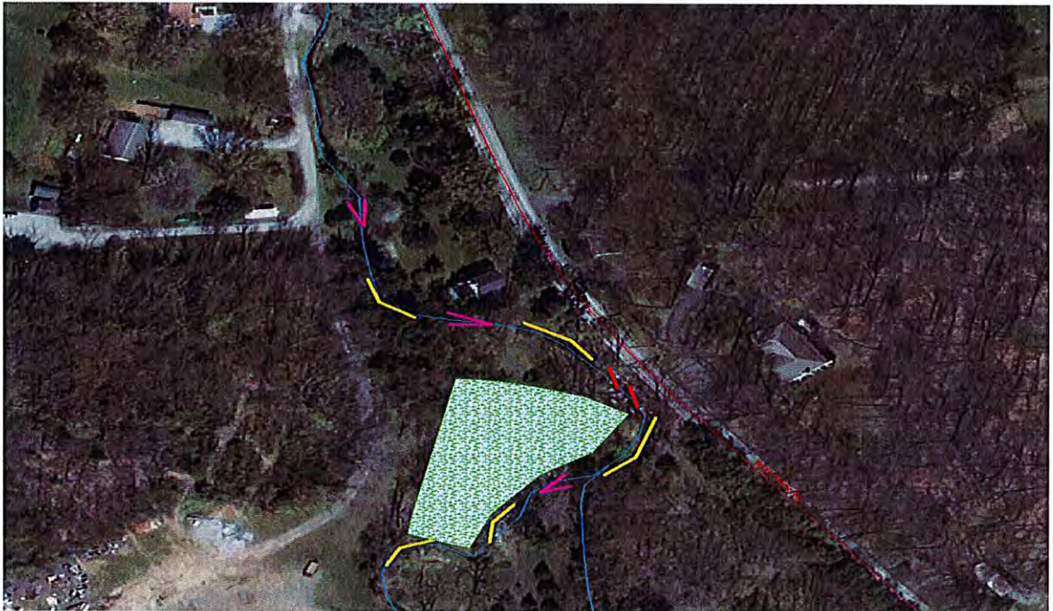
Yellow – mudsill, Pink – cross vane, Red – log vane, Teal – zig-zag wall, Green/Blue - buffer
