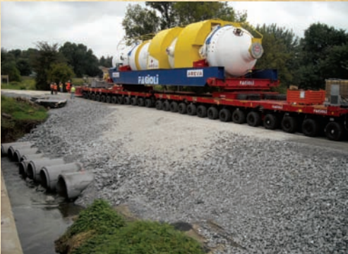
TMI Convoy crossing Pequea Creek with intermediate erosion controls.
